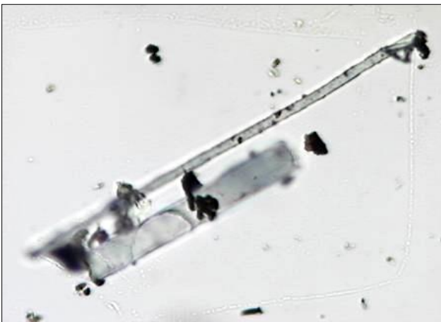
Sound liner fiberglass from HVAC system mixing box (optical microscopy)- 600x
