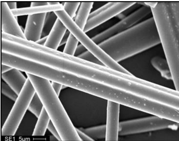
Owens Corning Pink insulation R-19 . High Na, moderate Ca glass
